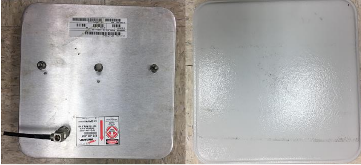
Figure 5.3 A photo showing the front side and back side of the RFID antenna.
